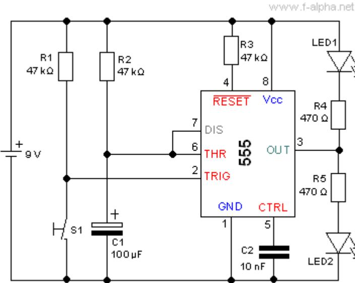
$$T = 1.1 \times R_2 C_1 \\ = 1.1 \times 47\,000 \Omega \times 0.0001 F = 5.2 \text{ sec}$$
